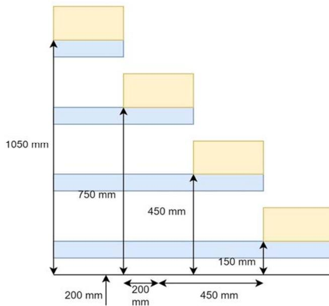
Provision of the first level (identified as "Level1") of a conveyor system consisting of two modular conveyors. These conveyors must allow easy rear fitting of a maximum of 4 levels, as shown in the figure below. The Maximum thickness of each conveyor must be 100mm. The maximum weight to be transported by the "Level 1" conveyor is 164Kg, distributed over its total length. The speed must be controllable from 0 to 0.5m/s independently for each conveyor.
